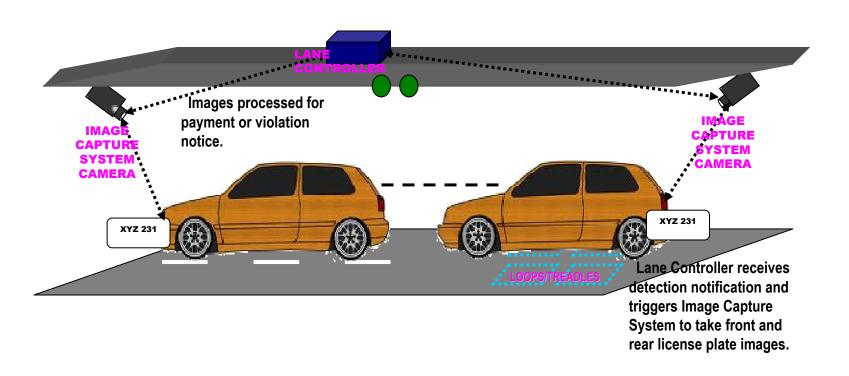
2. The loops prompt the lane controller to trigger the image capture system cameras to take rear and front license plate images. The images are then sent to the lane controller for processing to determine if a valid tag read has occurred.
